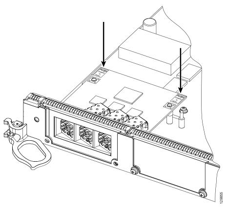
Figure 12 Rear Outer Corners of the EPA (Close-up)
